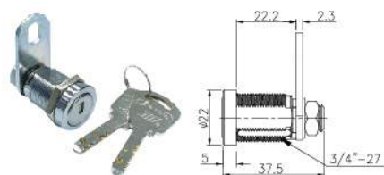
■ NC930 9 pin tumbler mechanism 10,000 combinations available
